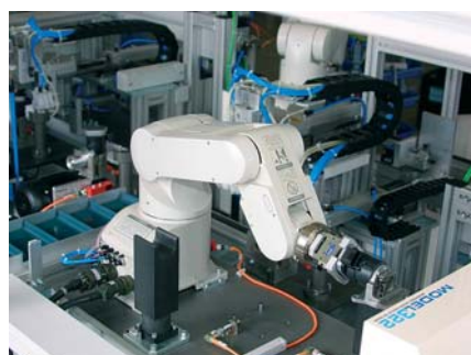
The RV-2SDB at work in typically cramped quarters
